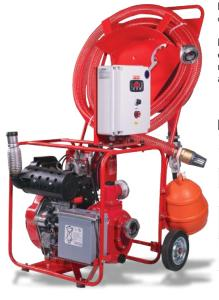
Portable diesel fire pump with self-priming, single-stage, horizontal type centrifugal pump directly coupled to a diesel engine provides the opportunity to intervene in fires at the initial stage.
