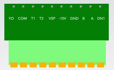
(1) Y0,COM. The internal circuit is shown below. Provide relay on/ off signal. Default meter detects device failure (you can control whether this function is disabled or not by bit5 of device\_config). Under normal conditions, the relay is closed. In case of fault, the relay is open.
